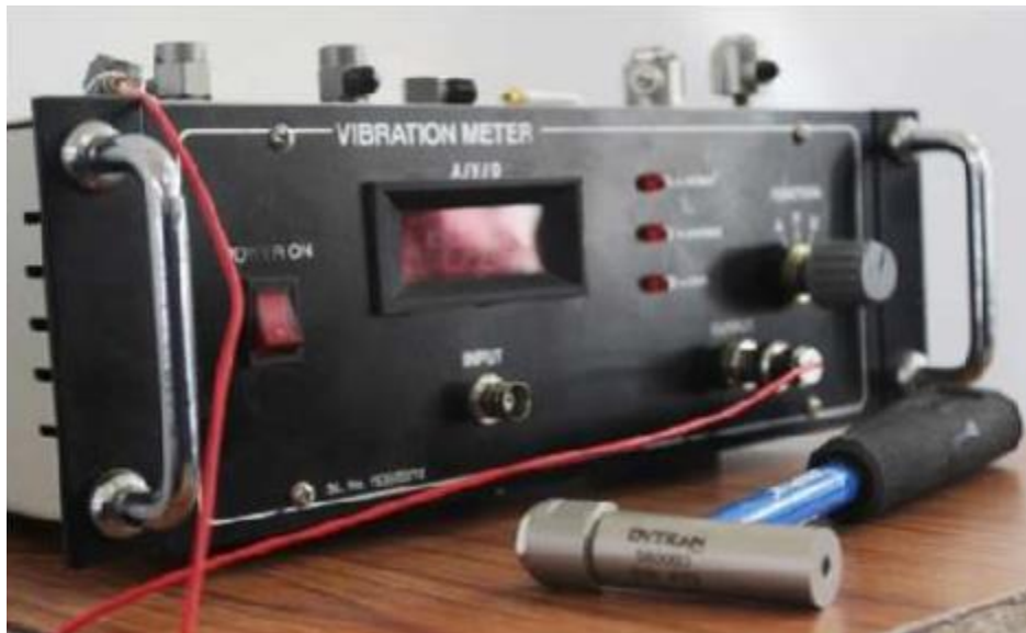
Fig. 3 Vibrometer, sensors, Impact hammer (LDS make, UK)
