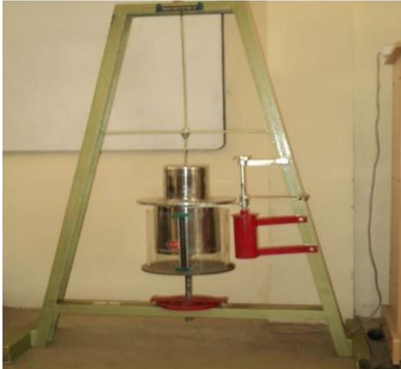
Fig. 6 Damped and undamped torsional vibration
