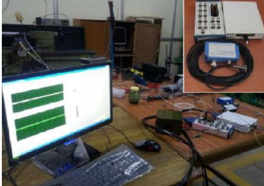
Fig. 4 Acoustic emission setup (Kistler make, Switzerland)
